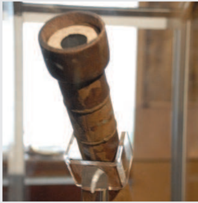
Fig. 7a: One of Galileo's two surviving telescopes came to the Franklin Institute in Philadelphia in 2009, on its first visit to the United States. Note that the outer part of the lens is covered with a cardboard ring. By hiding the outer part of the lens, which was the least accurate part, Galileo improved the quality of his images. (Photo: Jay M. Pasachoff).
